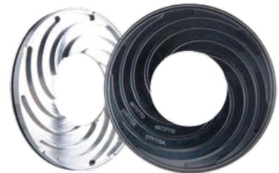
The double-sided spiral groove design of the TwisTorr stators combines centripetal and centrifugal pumping action in series, reducing considerably the size of the drag section and optimizing performance.
